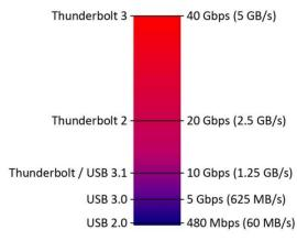
In Thunderbolt 3 mode, up to four lanes of PCIe Gen3 is supported for a maximum rate of 32 Gbps (4 GB/s); making it an ideal match for optimal data transfer performance of high-speed GaGe PCIe Gen3 Digitizers to connected PC devices.
